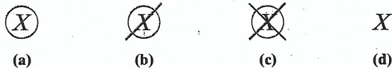
FIGURE 8-12 "Road" signs on a priority list. (a) Task X is ready. (b) Task X is in execution. (c) Task X is completed. (d) Task X is ineligible.
